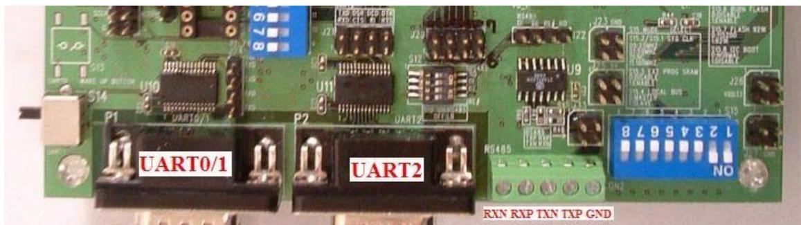
Figure 14. AX11015/AX11025 128-pin Development Board UART 0 Interface
