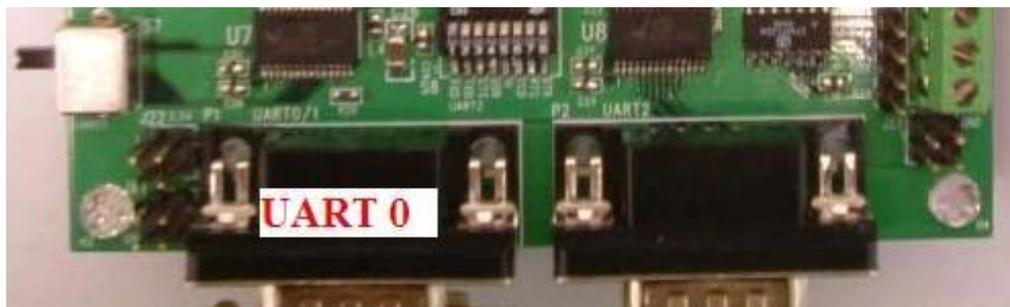
Figure 13. AX110xx 80-pin Development Board UART 0 Interface
