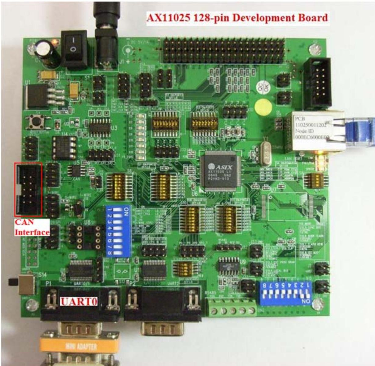
Figure 3. AX11025 128-pin Development Board
