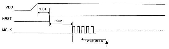
Reset of internal circuits is completed
