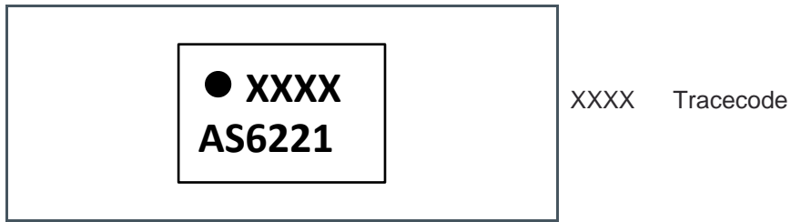
Figure 39: WLCSP Package Marking/Code for AS6221
